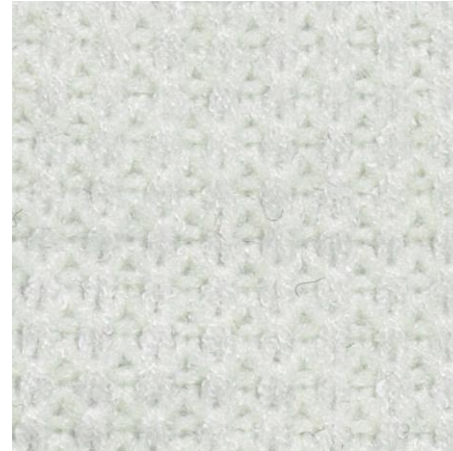
DIAMOND JERSEY KNIT COLOR OFF WHITE 50% Polyester / 30% Nylon / 20% Viscose Weight: 300 gsm | Width: 150 cm
